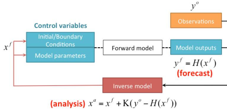
Figure 7: Data assimilation flow chart for a typical data-driven model.
