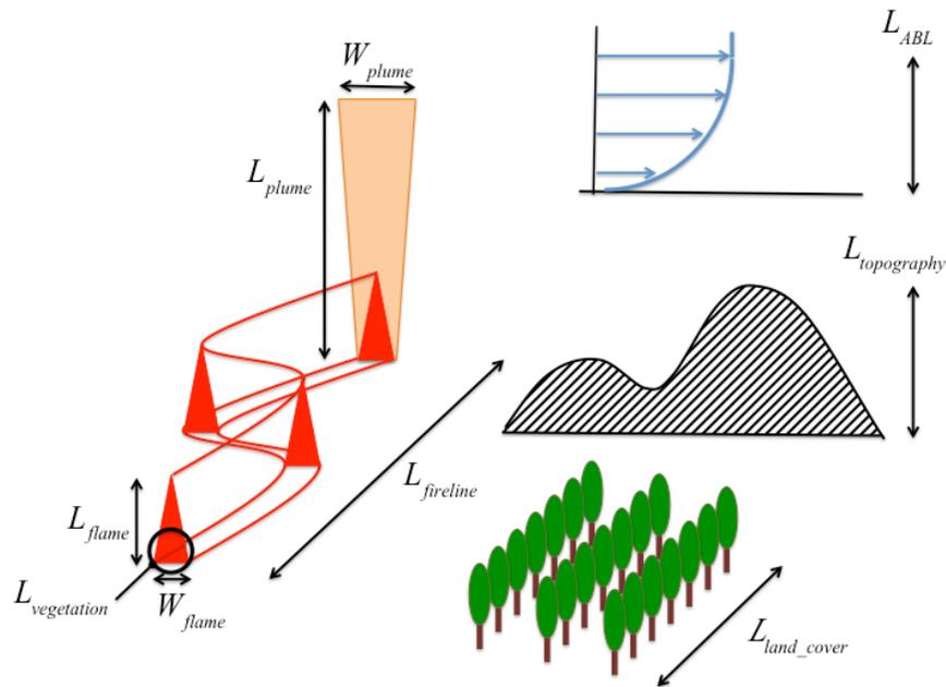
Figure 4: The different length scales that contribute to determining wildfire behavior: vegetation scales, flame scales, fireline scales, geographical scales (i.e. topographical scales and land cover scales) and meteorological scales.
