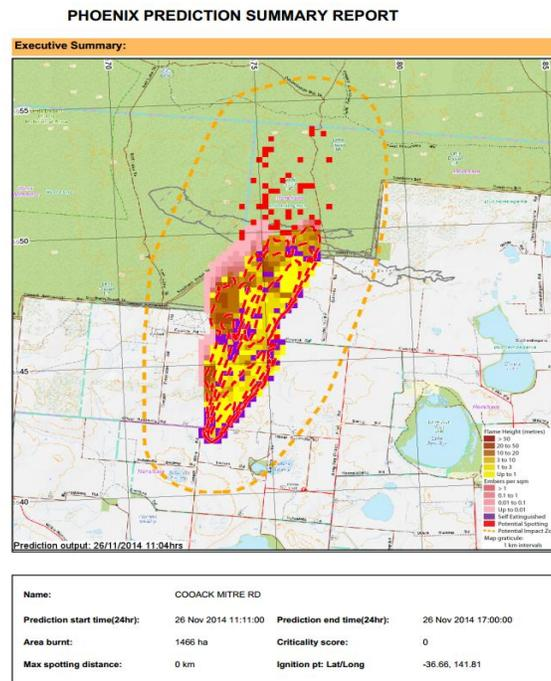
Figure 1: PHOENIX Rapidfire automated prediction report showing an estimate of the fire location (dotted orange line) and intensity, at a given time, through an ensemble of simulations that accounts for uncertainties in ignition location and timing [28].
