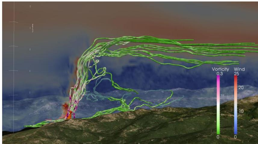
Figure 3: Illustration of current coupled fire-atmosphere capabilities: instantaneous snapshot from a mesoscale (several tens of kms) wildfire simulation using Meso-NH/ForeFire. The three-dimensional image shows wind speed in red/blue colors in a vertical slice along with vorticity in green/purple colors along spaghetti-like streamlines (the streamlines are positioned in the vicinity of the fire plume). Picture taken from Ref. [31].
