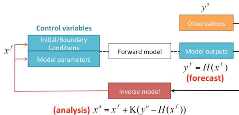
Figure 7: Data assimilation flow chart for a typical data-driven model.
