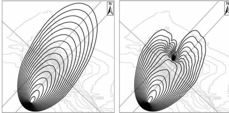
Figure 6: Simulation of wildfire spread using FARSITE with uniform wind (left picture) versus spatially-resolved wind (right picture). Reproduced from Ref. [44].
