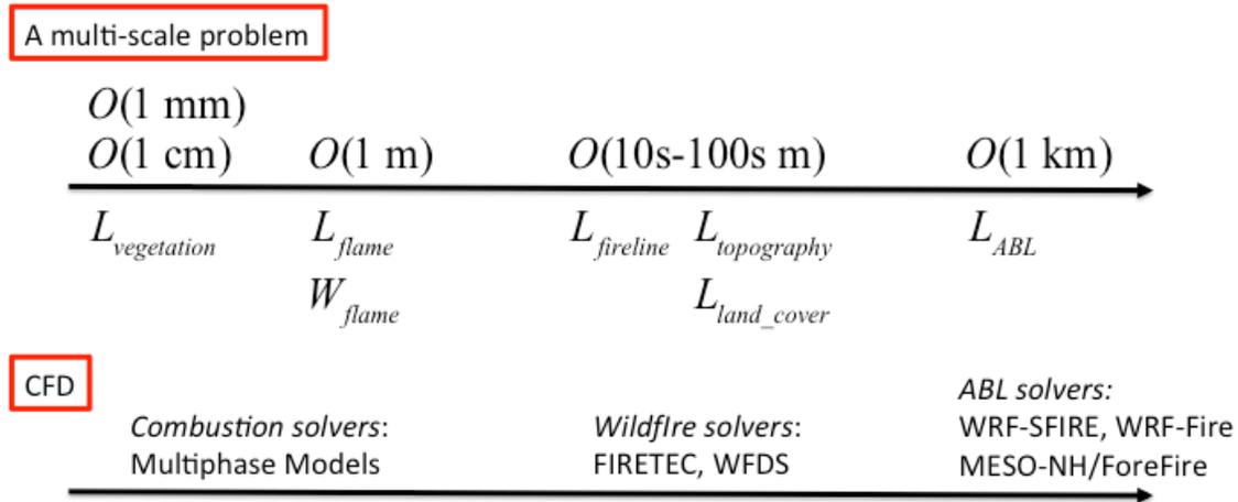
Figure 5: The different classes of CFD models used for wildfire spread simulations: combustion solvers resolve dynamics at the vegetation and flame scales; wildfire solvers resolve dynamics at the fireline and geographical scales; atmospheric boundary layers (ABL) solvers resolve dynamics at the meteorological scales.
